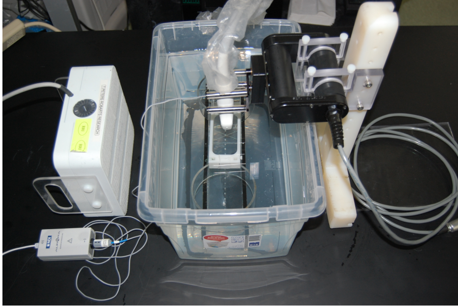
Figure 3.6: Experimental calibration setup comprising a magnetic tracking system, tracked ultrasound probe, tracked Z-bar calibration phantom, and plastic supports.
