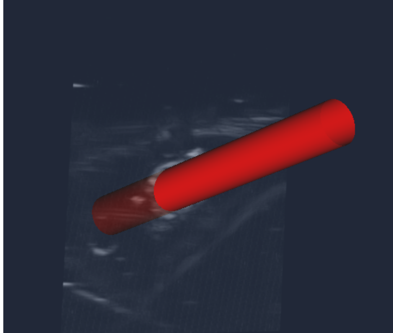
Figure 3.10: Visual representation of the straw phantom registered to the ultrasound image after calibration.
